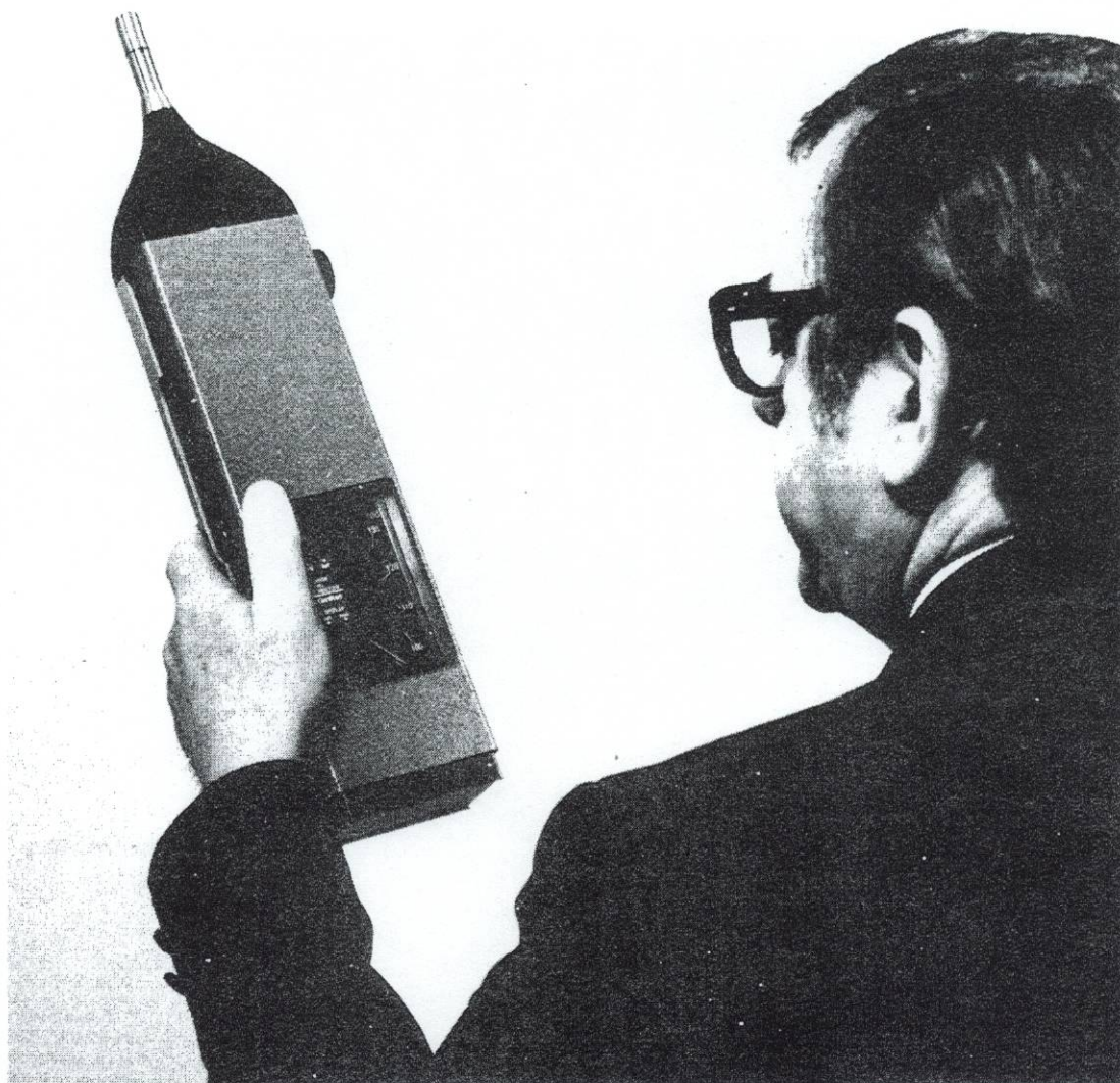
Figure 1-13. Random Response Microphone in Use
